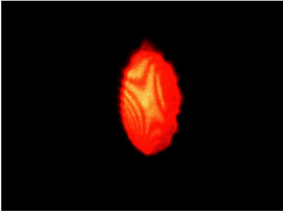
When a candle is placed underneath the air the beam is traveling through, the waves travel differently and create varying fringe patterns, as seen in the video
