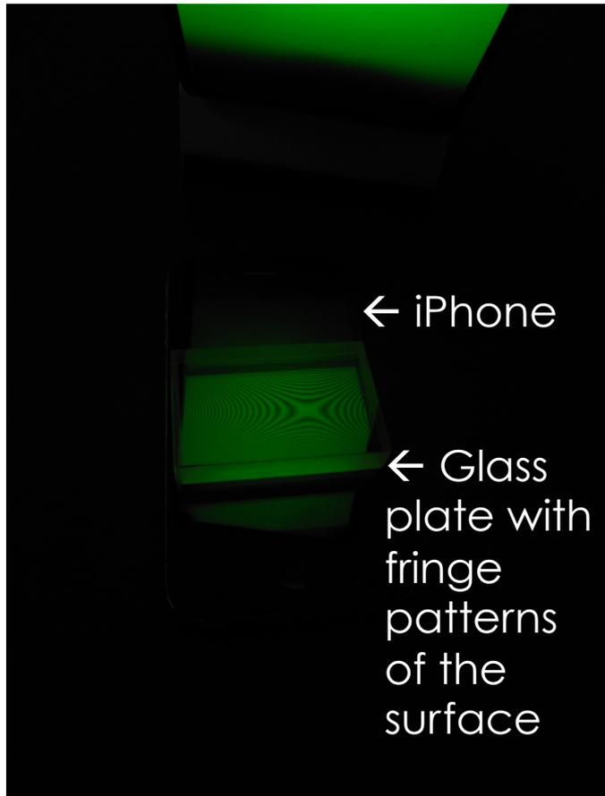
Using the same principles as the previous experiment, we used the screen of an iPhone as the second surface and determined just how flat the screen of an iPhone is.
